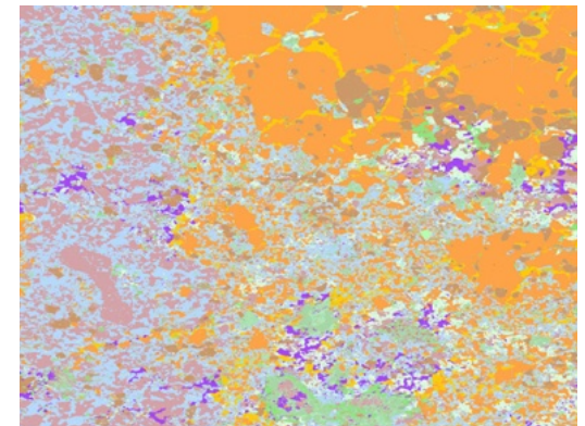
High resolution mineral map. Ni-Cu ore, Fraser Mine, Sudbury. Courtesy: University of Leicester, UK
