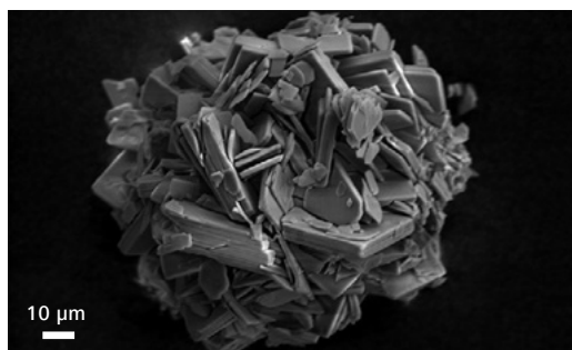
C2D imaging with drastically reduced charging effect (Sample: Lanthanum carbonate, a phosphate binder used as a oral therapeutic agent for dialysis patients.).
