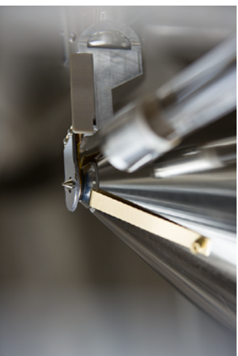
Retractable NanoVP differential pumping aperture inside the SEM chamber.
