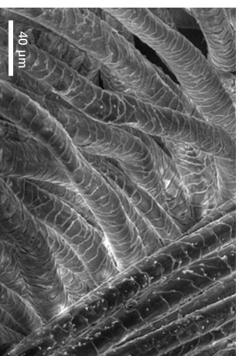
Silver nanoparticle coated natural fibers imaged with NanoVP at 80 Pa, at 10 kV. Sample: courtesy of F. Simon, Leibniz-Institute for Polymer Research Dresden e.V., Germany.
