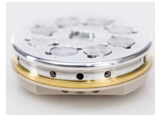
Tandem decel sample holder for 9 single specimens.
